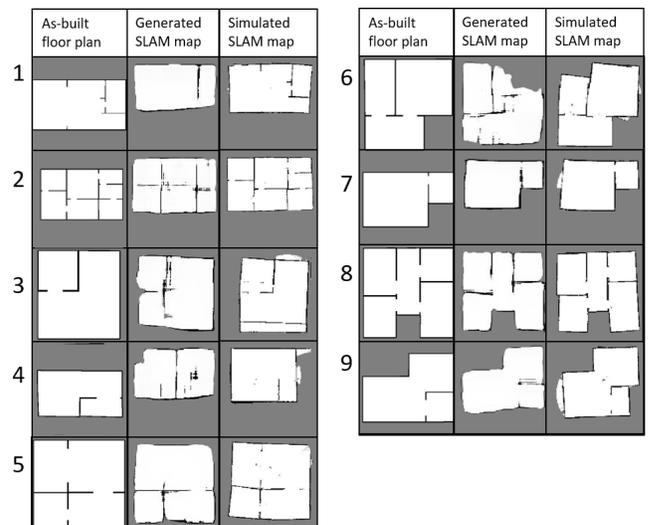
Fig. 7. Test results of  $Model_{AB}$
